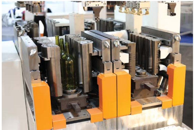
This 1-section ISX 6 1/4in triple gob and 4 1/4in quad gob equipment was exhibited at glasstec 2018.
