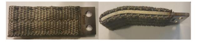
4. Ceramic coating – on the stainless steel carrier is a sprayed ceramic coating up to a maximum thickness of 1 mm
