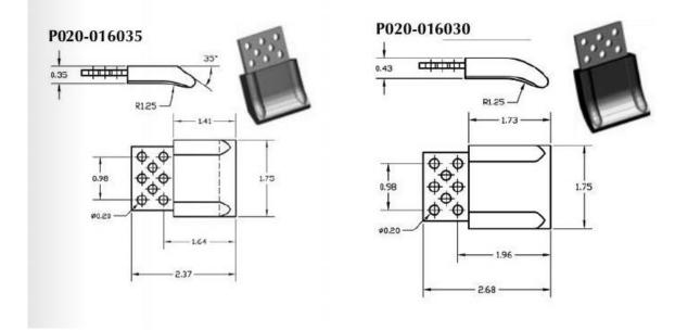
2. Graphite composite - graphite composite with oriented carbon fibers in the form of a fabric, the blanks are plate-shaped. Supplied by f. Pyrotek, Duratemp further used on Fingers with air pocket
